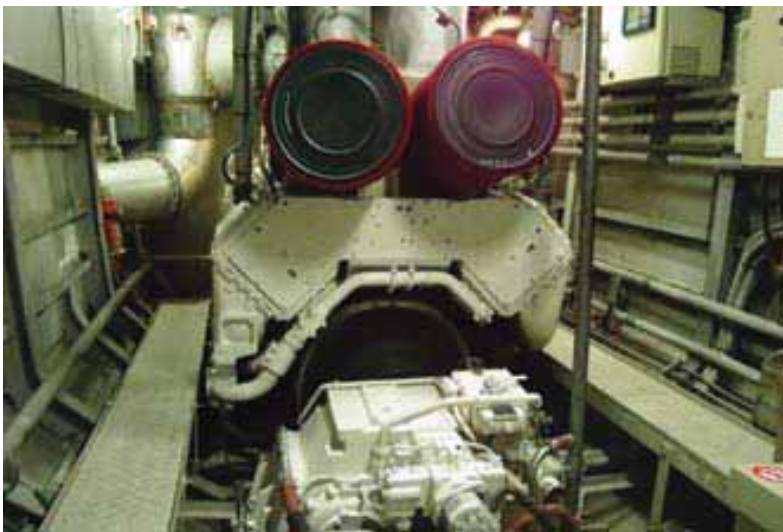
A 2000 kilowatt diesel engine – main propulsion for a high speed ferry.
