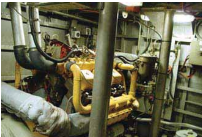
An auxiliary diesel engine such as this one may also be present in the engine room. It drives a 240 generator powering refrigeration, air conditioning, lighting and other appliances common on today's commercial ships. Care must be taken when working in a machinery space, as hot surfaces, moving machinery and a great deal of noise make this a hazardous environment at sea. Always wear appropriate PPE.
