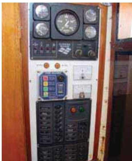
A DC circuit breaker panel on a small commercial vessel. Fire alarm, warning lights, engine instruments, voltmeter and ammeter are also incorporated. A separate panel exists for the AC system.
