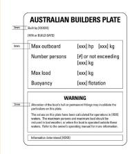
\* This is a sample of an ABP for a boat less than 6 meters with an outboard motor.
