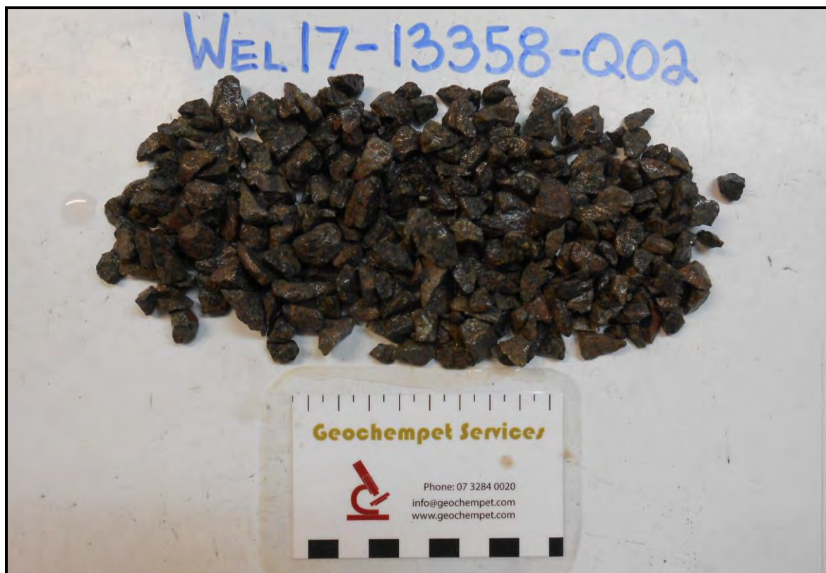
Plate 1: Photograph of a washed sub-sample of the supplied 10 mm aggregate.
