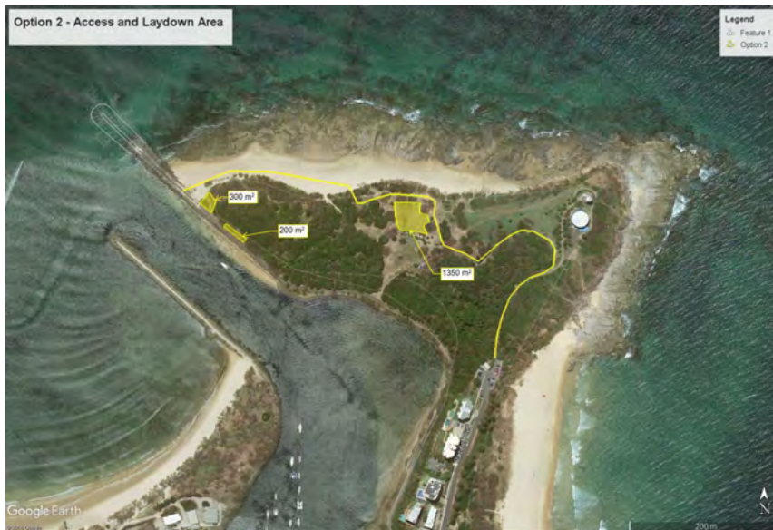
Figure 4.6 Option 2 land-based vehicle access and potential laydown areas.
