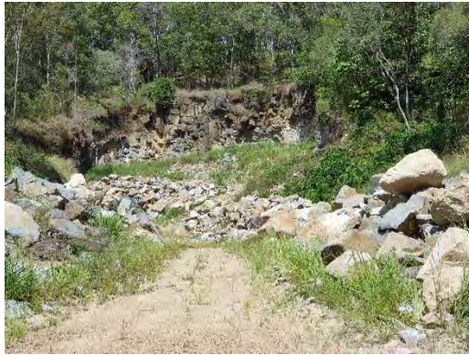
Figure 1.2 Kuluin Quarry from fence-line (15 March 2019). Estimated rock D_{50} is approx. 1.2 m.
