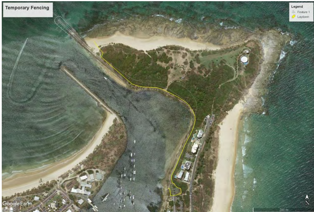
Figure 4.2 Minimum requirement for temporary fencing for land-based construction along eastern bank of Mooloolah River. Total length is 800 m.
