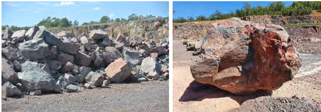
Figure 2.2 Left: stockpile of Glass House Quarry armour rock with estimated D_{50} of 0.75 m. Right: large boulder ( D_{50} approximately 1.7 m).
