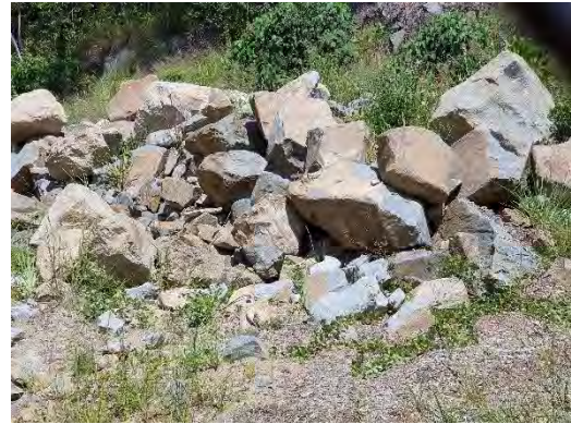
Figure 1.2 Kuluin Quarry from fence-line (15 March 2019). Estimated rock D_{50} is approx. 1.2 m.
