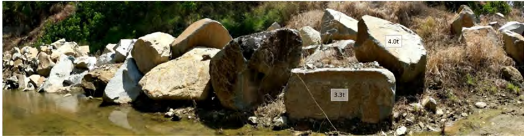
Figure 4.3 Panoramic view of Stockpile W-2 (Western area) showing large armourstone (up to 4t approx.)
