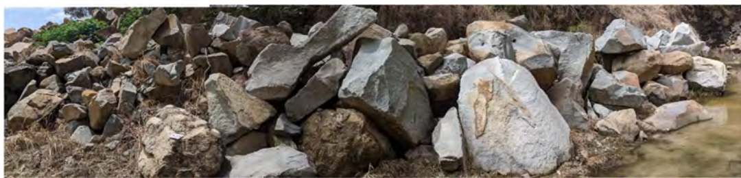
Figure 4.2 Panoramic view of E-2 Stockpile (Eastern area) showing widely graded rock (approx. 15 kg to 40kg rock to the left and approx. 0.8 to 2.4t rock toward the right)
