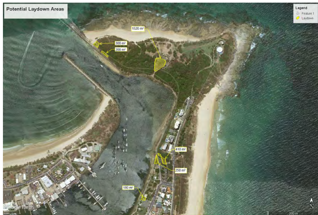
Figure 4.4 Identified clearing areas for use as potential laydown areas, stockpiling or turn-around areas for land-based construction
