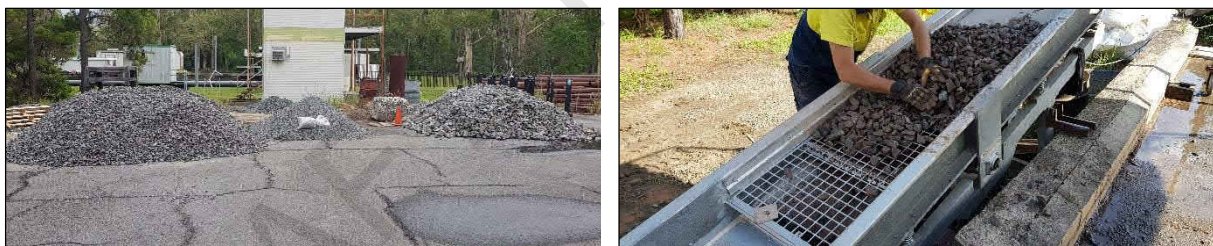
Figure 4: Example photos of rock sorting. Raw stock rock piles (left); sieve fractionation of model rock (right).
