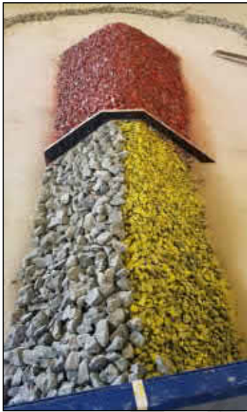
Figure 15: Photos depicting the installation of the core (top) and armour layers (bottom left) using templates. The footprint of the breakwater layers was drawn on the concrete floor as shown in the bottom right picture.
