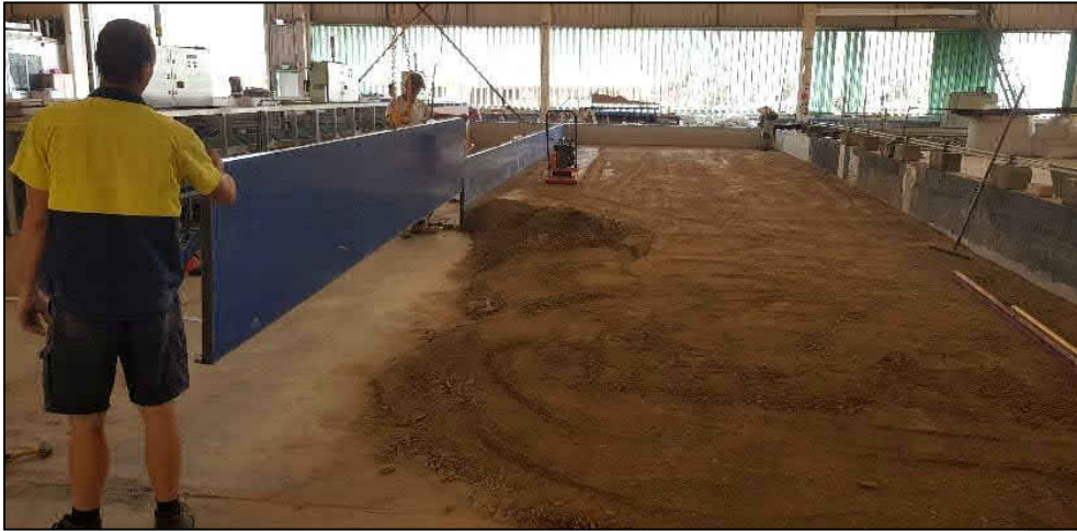
Figure 10: Flume bathymetry construction - supporting walls installation, road base fill and compaction progressing.
