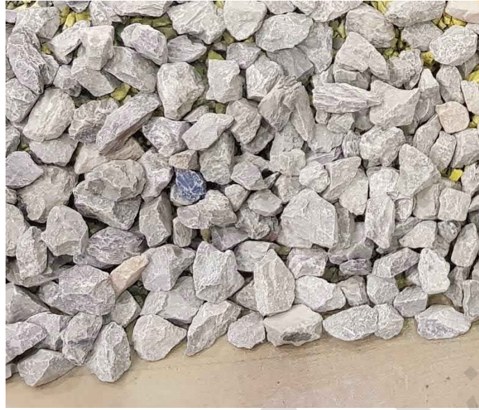
Figure 6: Example of Armour rocks used.
