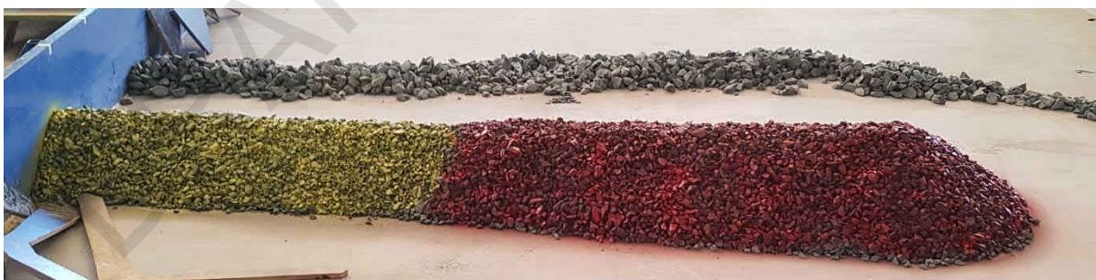
Figure 8: Example of core (yellow) and filter rocks (red).
