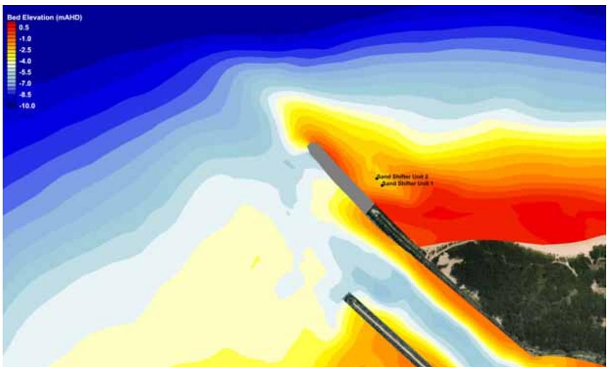
Figure 7-5 Option 3 with Sand Shifter Bed Elevation at the end of Assessment Period
