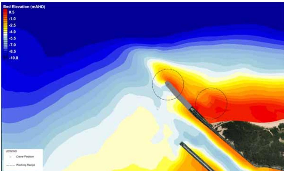
Figure 7-11 Option 3 90t Crawler Crane Positions and Working Ranges used to Estimate Bypass Volume
