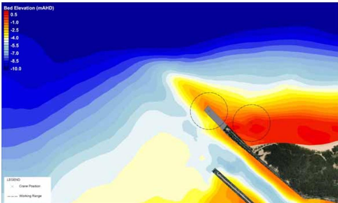
Figure 7-13 Option 3b 90t Crawler Crane Positions and Working Ranges used to Estimate Bypass Volume
