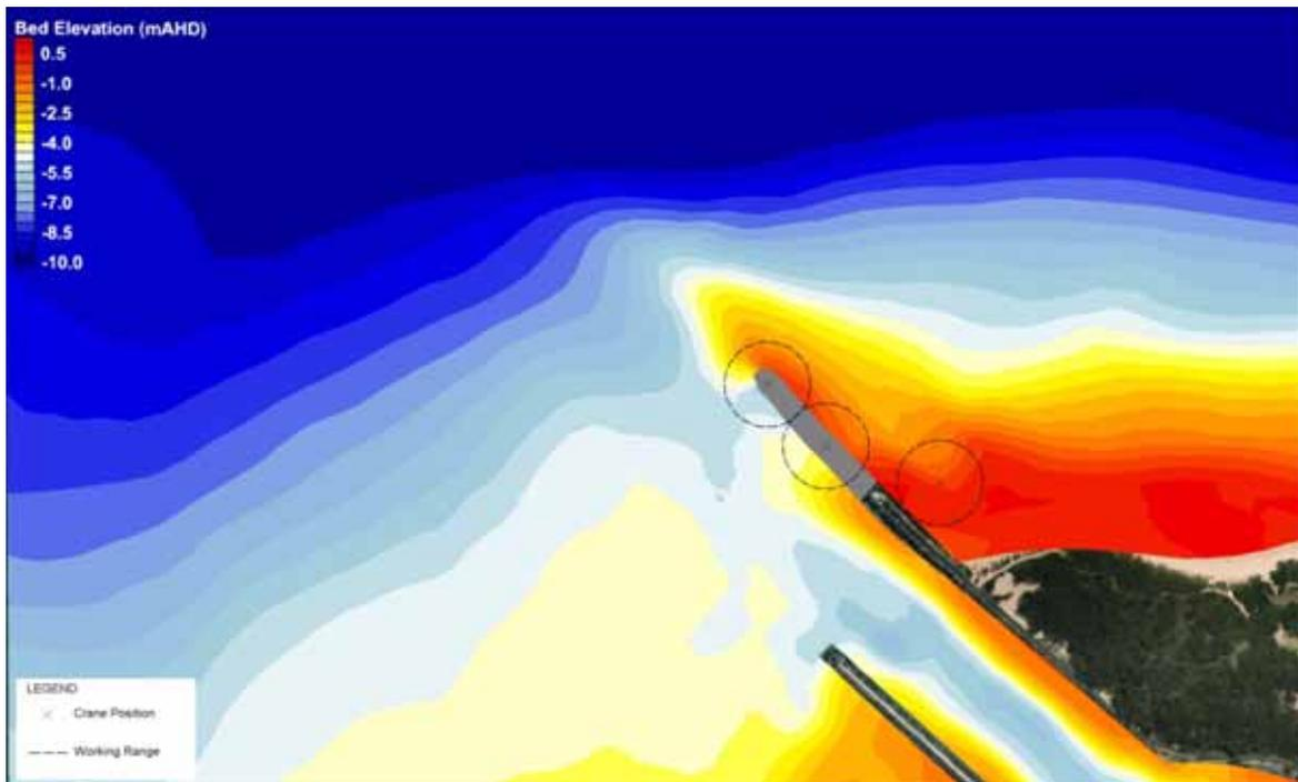
Figure 7-10 Option 3 50t Crawler Crane Positions and Working Ranges used to Estimate Bypass Volume
