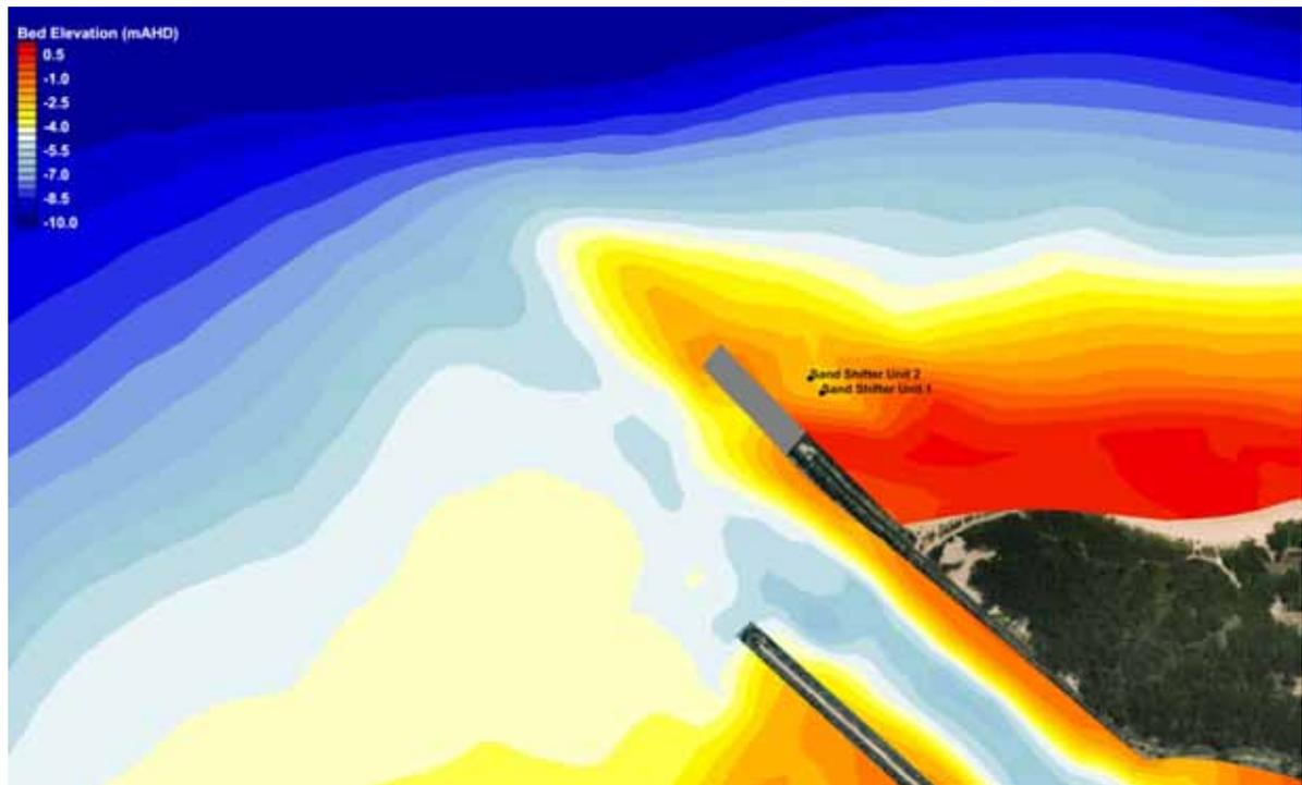
**Figure 7-6 Option 3b with Sand Shifter Bed Elevation at the end of Assessment Period**
