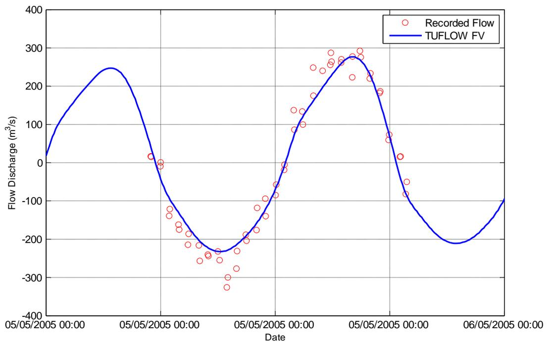
Figure 3-5 ADCP Flow Comparisons from May 2005 Monitoring
