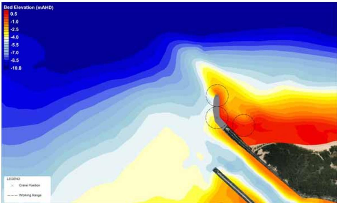
Figure 7-8 Option 2 50t Crawler Crane Positions and Working Ranges used to Estimate Bypass Volume
