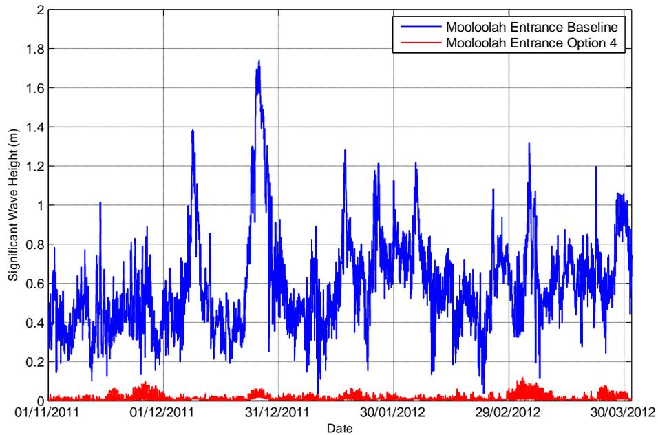
Figure 4-30 Option 4 and Baseline Harbour Entrance Significant Wave Height Time Series Comparison
