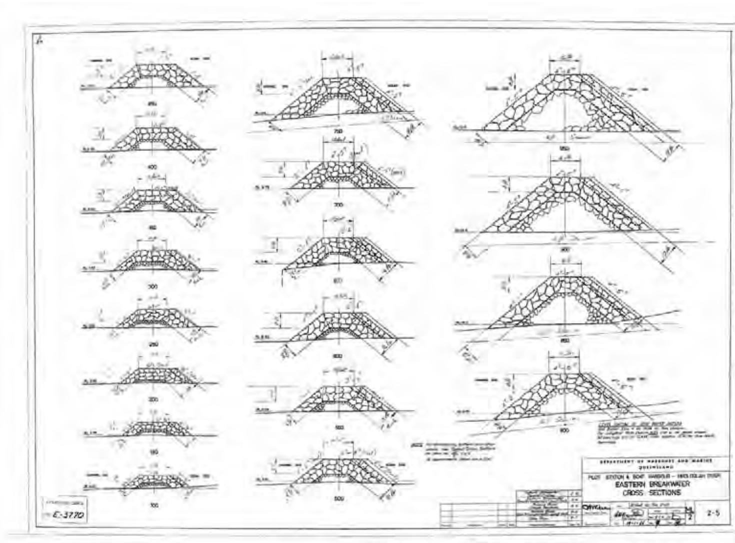
Figure 6-2 Existing Eastern Breakwater Cross Sections (provided by TMR)
