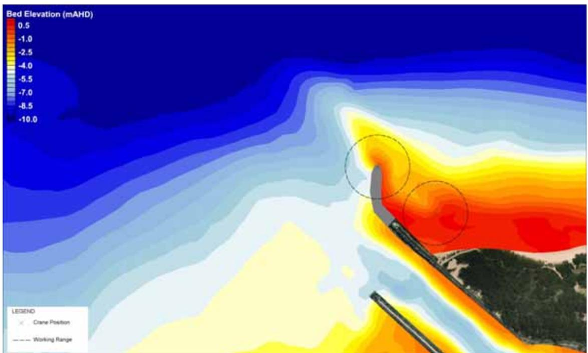
Figure 7-9 Option 2 90t Crawler Crane Positions and Working Ranges used to Estimate Bypass Volume
