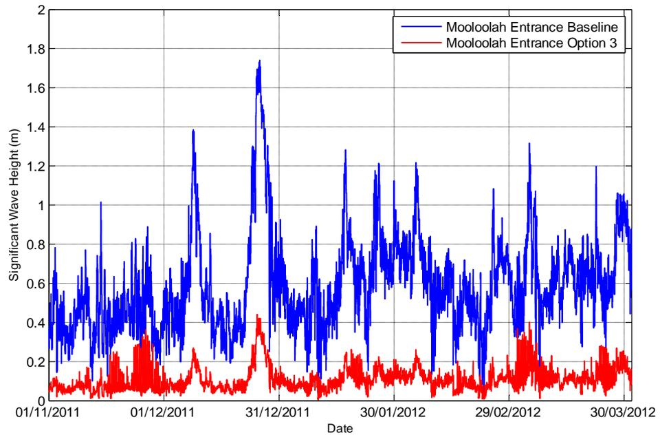
Figure 4-23 Option 3 and Baseline Harbour Entrance Significant Wave Height Time series Comparison
