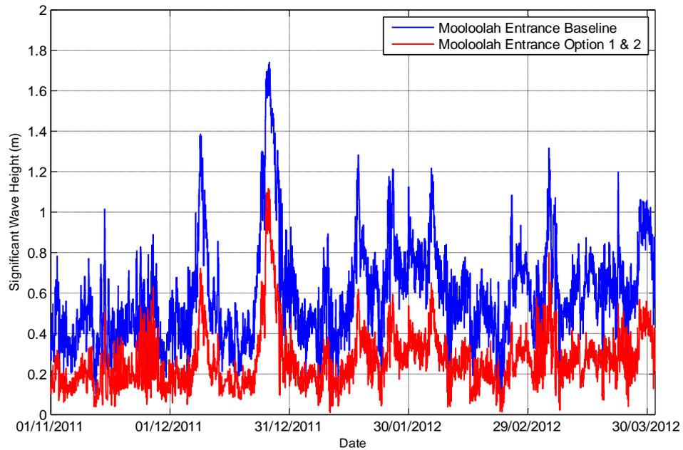
Figure 4-16 Option 1 & 2 and Baseline Harbour Entrance Significant Wave Height Time series Comparison
