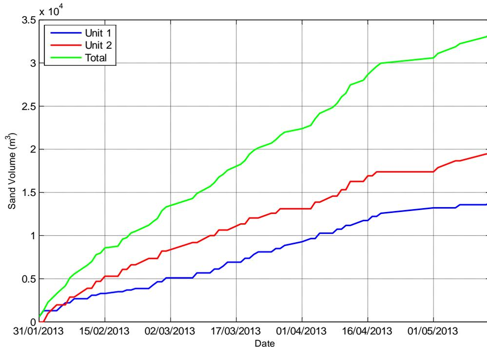
Figure 7-3 Noosa Main Beach Sand Shifter System Production during 2013 (Slurry Systems Marine)
