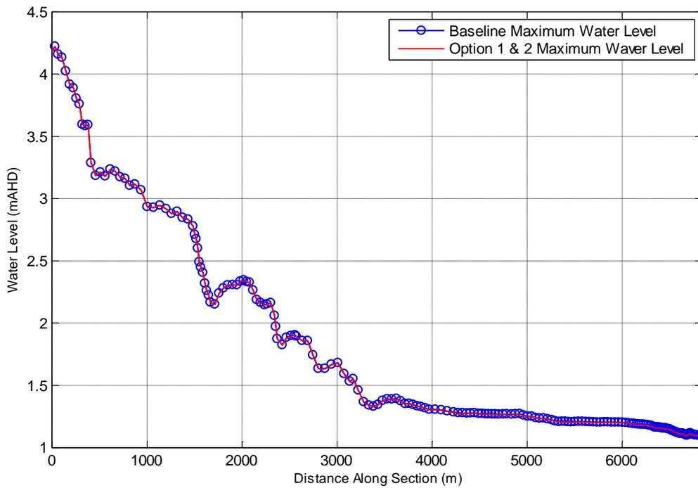
Figure 4-21 Option 1 & 2 and Baseline Flood Assessment Maximum Water Level Comparison
