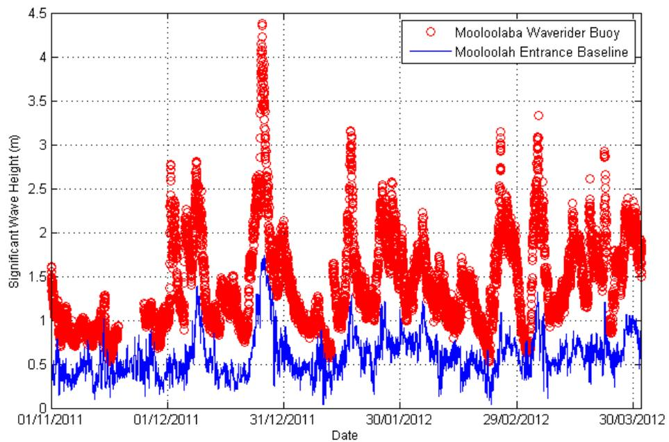
Figure 4-8 Offshore and Baseline Harbour Entrance Significant Wave Height Time series Comparison
