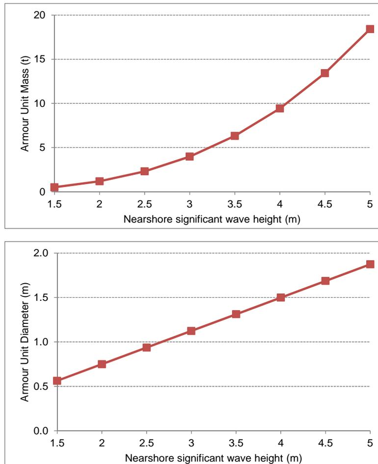
**Figure 6-3 Relationship between Armour Stone Characteristics and Significant Wave Height – 2:1 Sloping Permeable Structure (Hudson 1953, 1959)**
