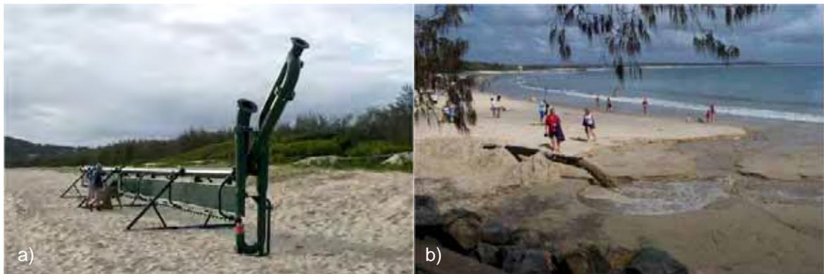
**Figure 7-2 Noosa Main Beach Sand Shifter System: a) Sand Shifter Unit before burial; b) Sand/Seawater Mixture Pumping (Slurry Systems Marine)**
