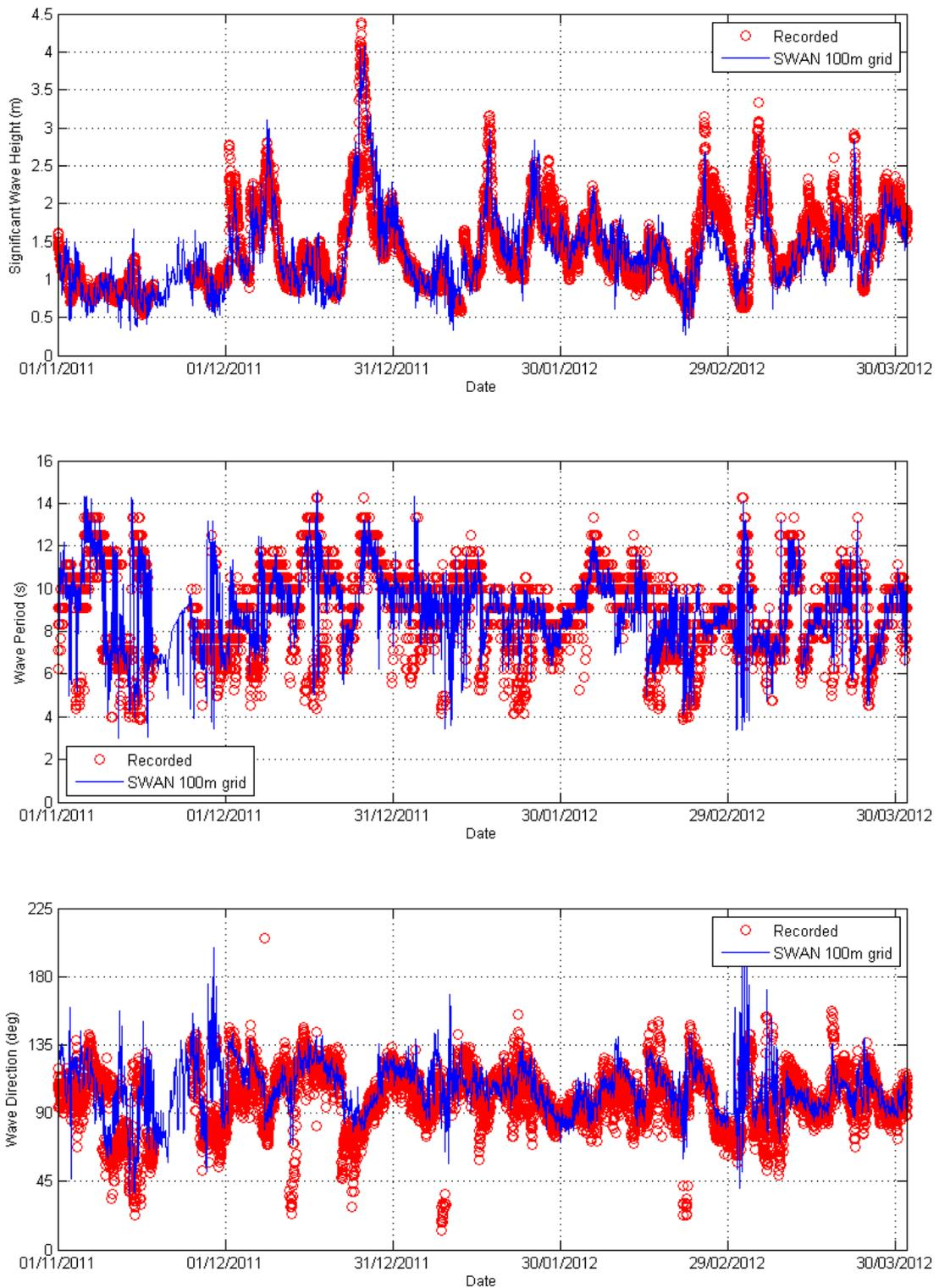
Figure 3-2 SWAN Model Validation to Mooloolaba Waverider Buoy Measurements
