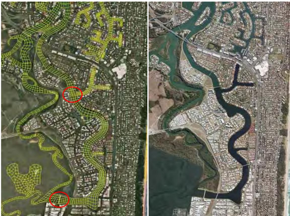
**Figure 3-3 Weir Locations Shown within TUFLOW FV Model Mesh (left) and Recent Aerial Photography Indicating Weir Closure (right)**
