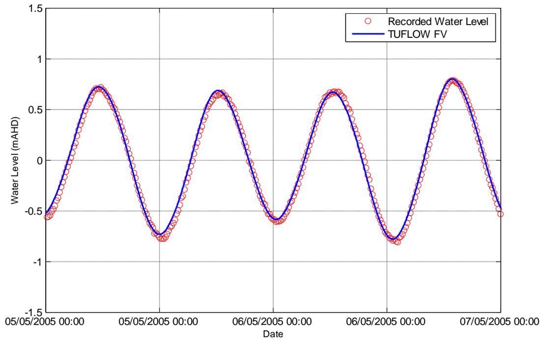
Figure 3-4 Tide Recorder Comparisons from May 2005 Monitoring
