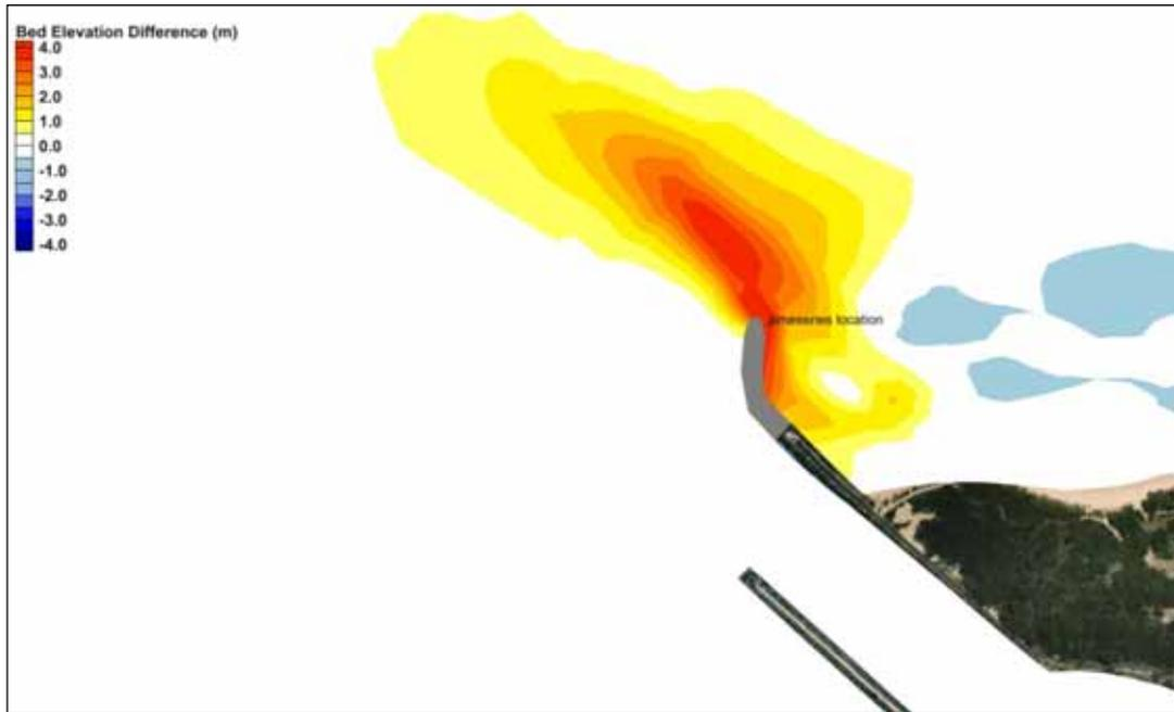
Figure 4-19 Option 1 & 2 Total Bed Elevation Difference
