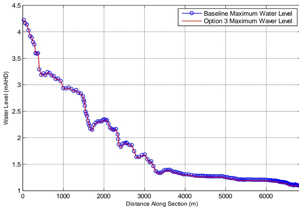
Figure 4-28 Option 3 and Baseline Flood Assessment Maximum Water Level Comparison
