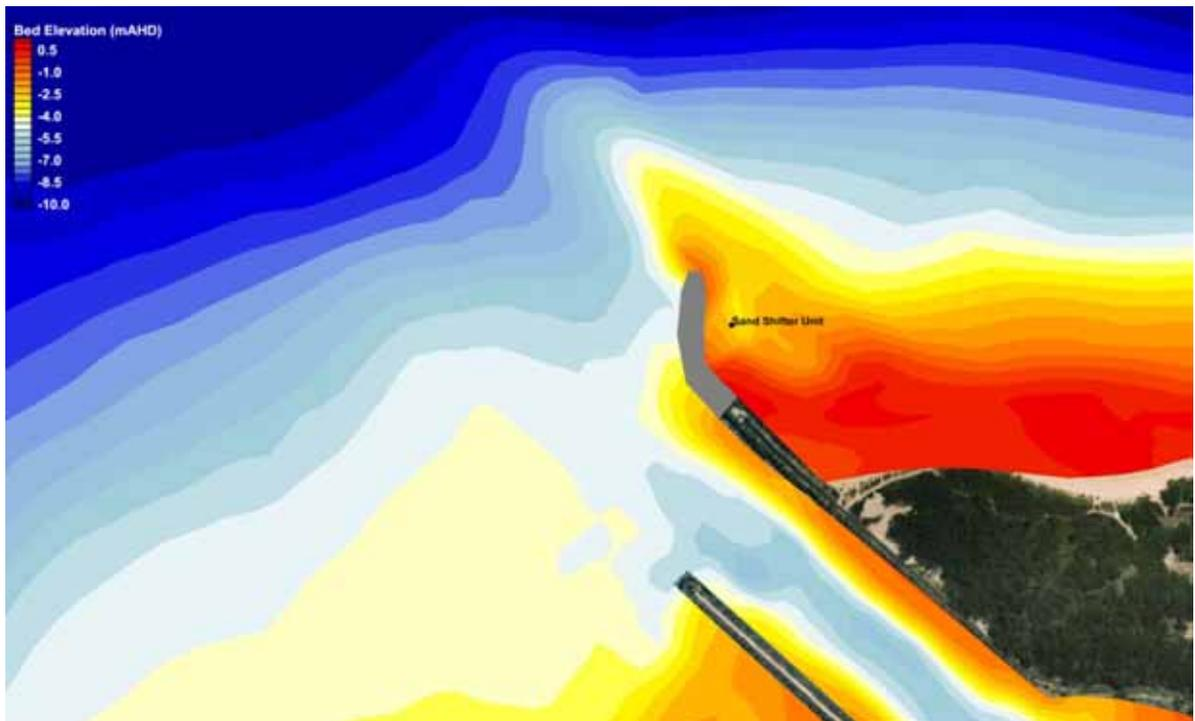
Figure 7-4 Option 2 with Sand Shifter Bed Elevation at the end of Assessment Period
