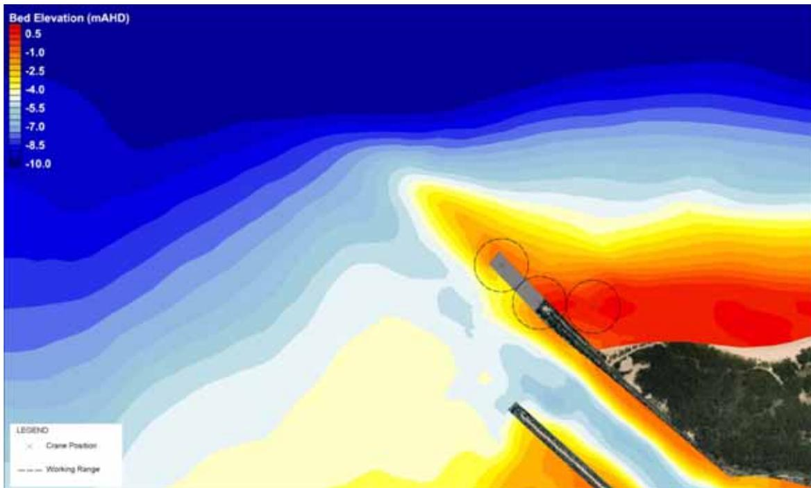
Figure 7-12 Option 3b 50t Crawler Crane Positions and Working Ranges used to Estimate Bypass Volume
