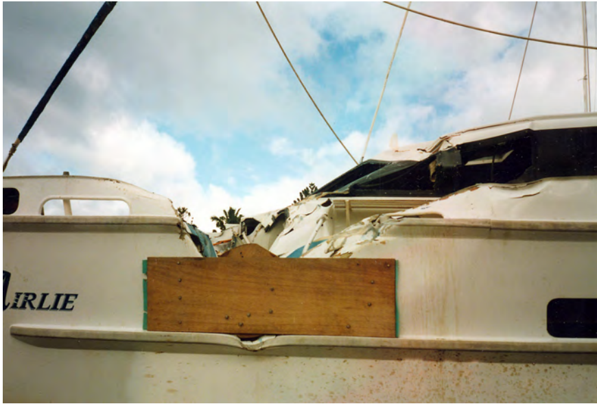
Photo 7 - The point of impact showing damage to the Pride of Airlie.
