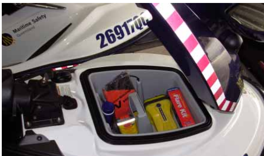
Figure 10: PWC with safety equipment in place
