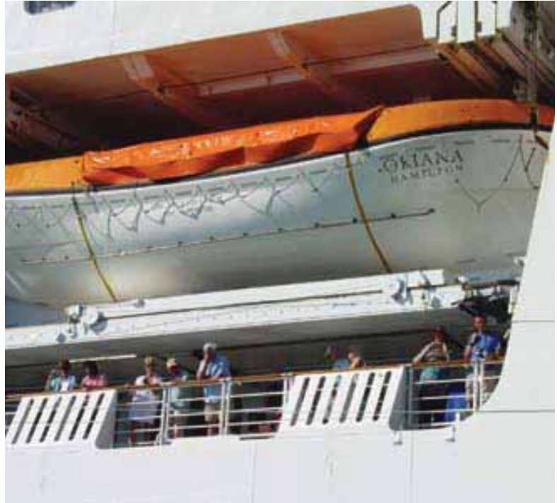
A class 1 passenger ship lifeboat stowed on extendable davits.
