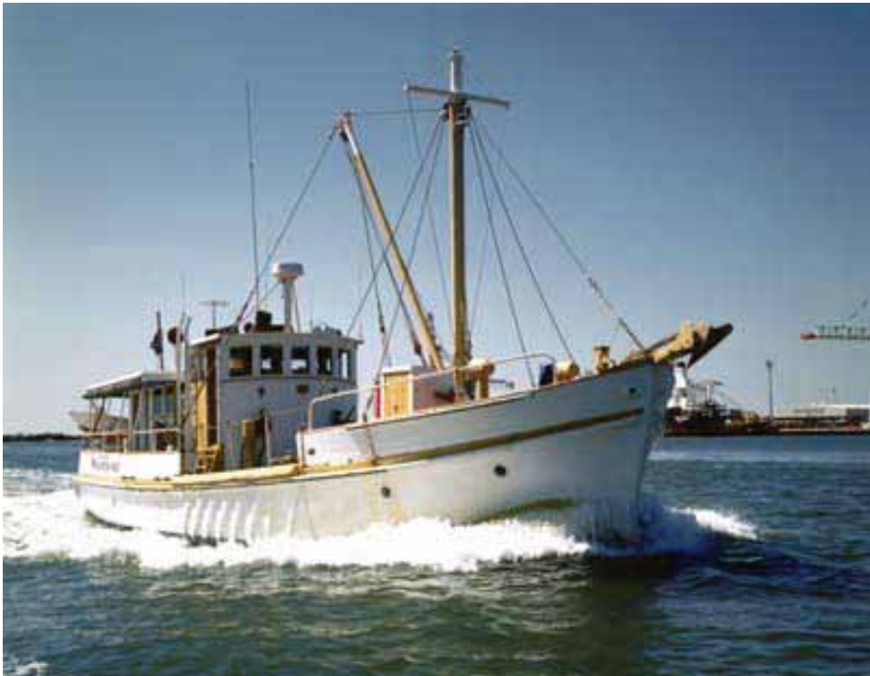
This vessel uses a derrick rather than a crane for handling cargo.
