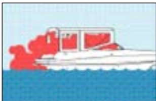
Inadequately ventilated canvas enclosures.
