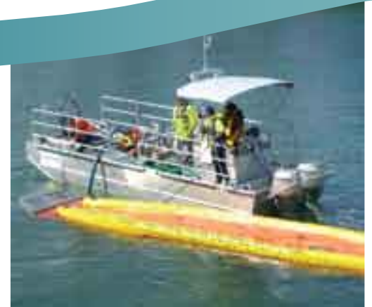
Testing of 20,000 litre capacity temporary storage bags in Auckland Harbour.
