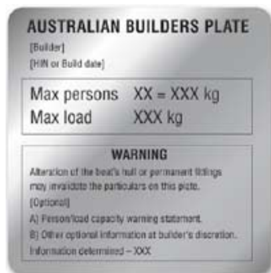
Above: example of an Australian Builders Plate for vessels greater than six metres.
