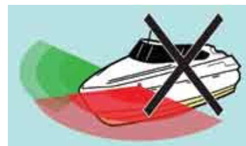
Incorrect installation – side lights.
