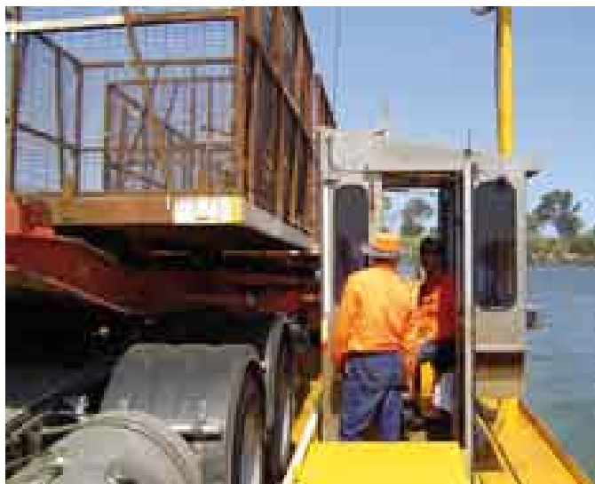
Cane bins obscured vision from the original cabin position.
