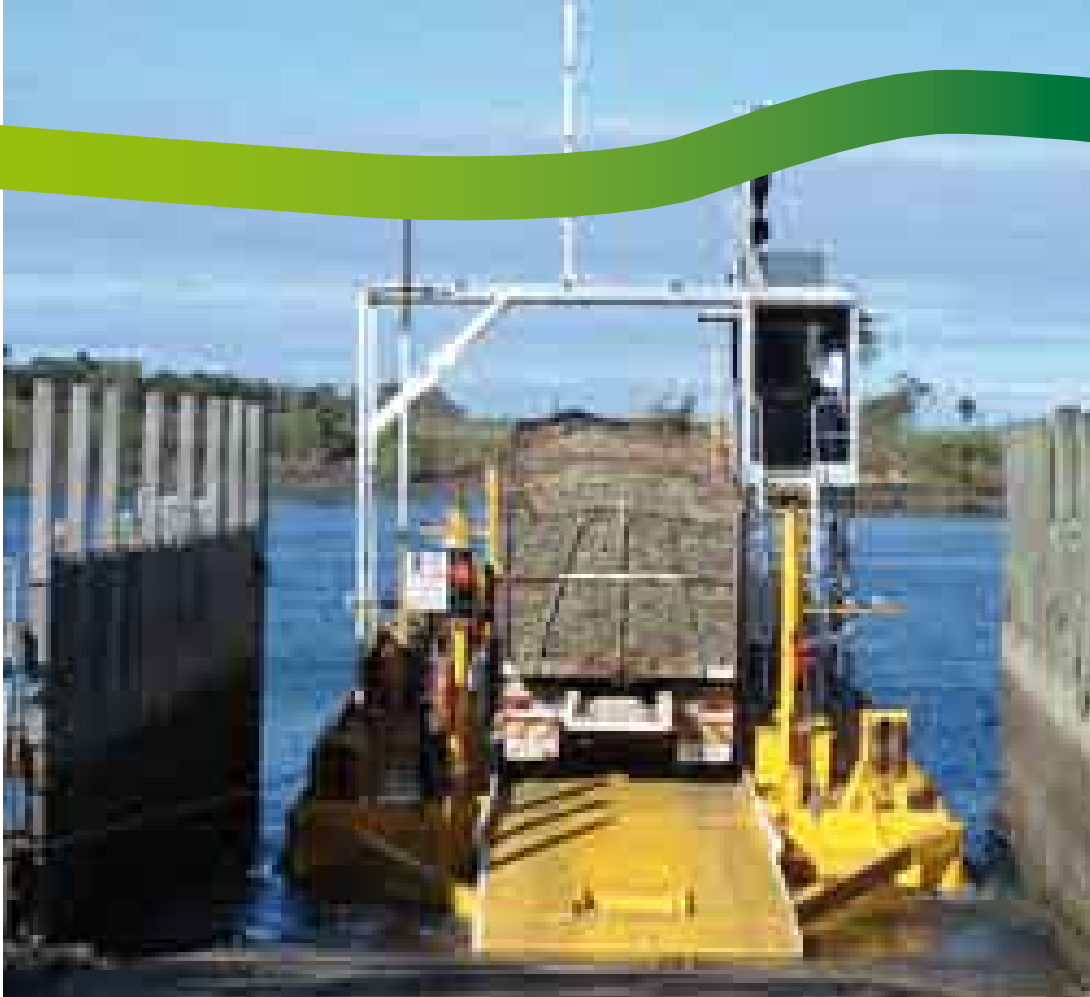
The new cabin positioned higher for increased visibility and safety.
