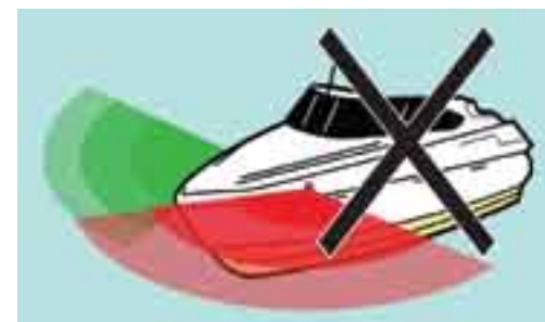
Incorrect installation – side lights.
