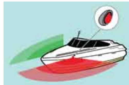
Correct installation – side lights.
