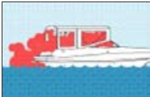
Inadequately ventilated canvas enclosures.
