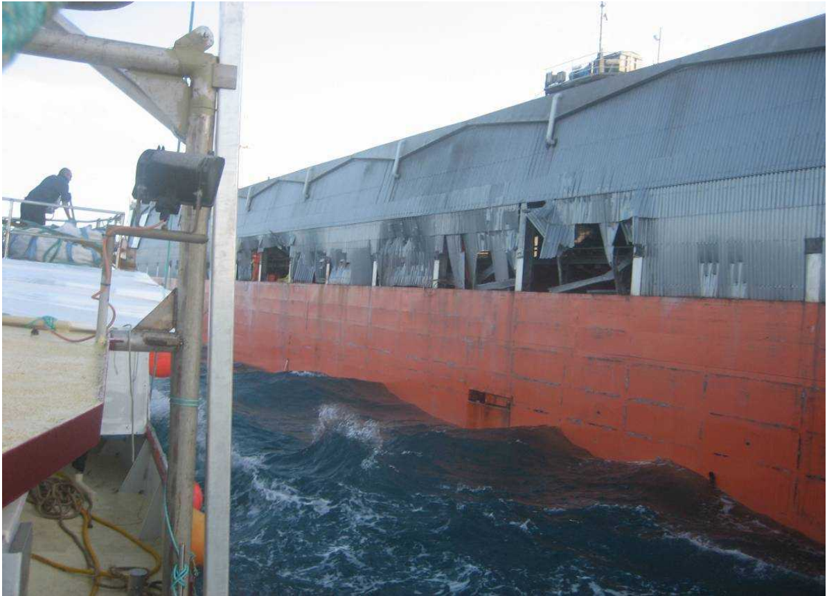
Figure 12 - Damage to the Canopy on the Port Side
