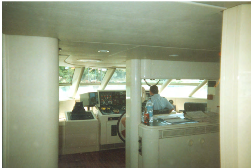
Photo 9 - The bridge of the Sun Paradise showing the intercom and access to the conning position.
