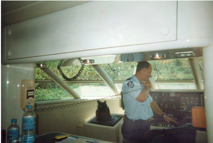
Photo 9 - The bridge of the Sun Paradise showing the intercom and access to the conning position.
